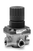
» Mod. VMR: maintains system pressure at a constant set point. In case of system, tank or line over-pressure state, will rapidly exhaust to atmosphere until set point is reached thereby closing off exhaust flow from the VMR relief valve
